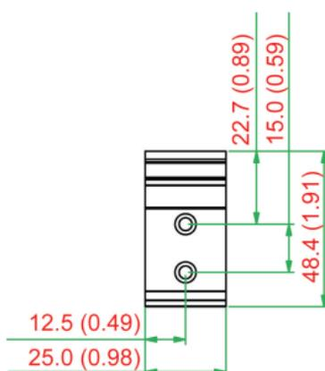
The OnCell G3150A-LTE Series computers come with a DIN-rail kit attached to the back panel. Mount the OnCell G3150A-LTE Series on corrosion-free mounting rails that meet the EN 60715 standard.
