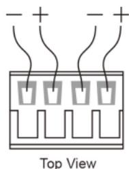
**STEP 1:** Insert the negative/positive DC wires into the V-/V+ terminals.
