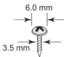
**NOTE** Test the screw head and shank size by inserting the screws into one of the keyhole shaped apertures of the wall-mounting plates before attaching the plates to the wall.
