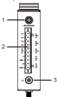
1. GPS antenna connector (female SMA)
