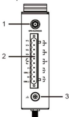
1. GPS antenna connector (female SMA)
