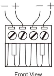
**STEP 3:** Insert the plastic terminal block connector prongs into the terminal block receptor, which is located on the top panel of the OnCell G3150A-LTE.
