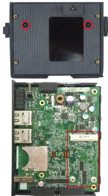
3. Remove the plastic plate and the sticker on both sides of the **large** thermal pad and place it in the socket. Press the thermal pad down so that it sticks to the base of the socket. Place the thermal pad as close as possible to the holes for the screws used to secure the module.
