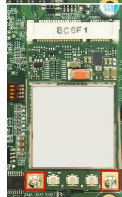
5. Remove the plastic plate and the sticker on both side of the **small** thermal pad and stick the thermal pad on to the module.
