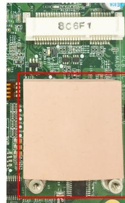
4. Insert the cellular module into the socket and tighten the screws to secure the module to the socket.
