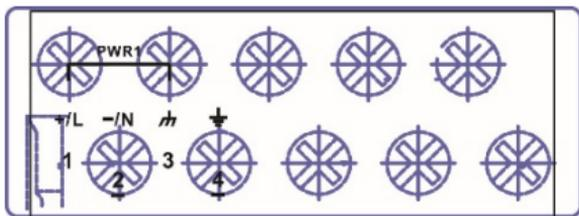
**STEP 1:** Insert the L/N AC wires into the PWR1 terminals (L → pin 1, N → pin 2).
