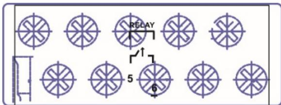
**FAULT:** The RELAY contacts of the 10-pin terminal block connector are used to detect user-configured events. The two wires attached to the RELAY contacts form an open circuit when a user-configured event is triggered. If a user-configured event does not occur, the RELAY circuit will be closed.
