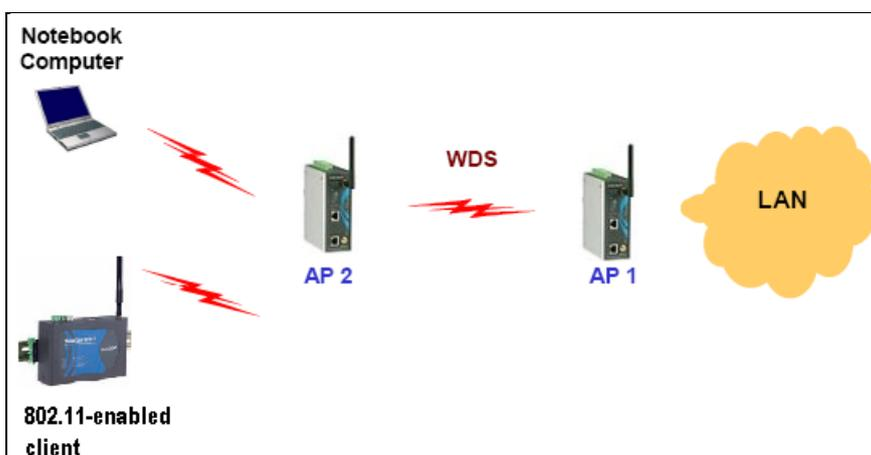
By using WDS, two or more LAN segments can be connected wirelessly. As illustrated in the figure below, a pair of wireless LAN-to-LAN bridges is used to connect two LAN segments. Since the AP is WDS-enabled, it can be used as a wireless bridge.
