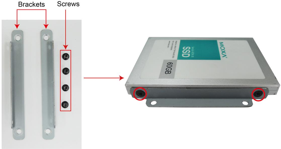
4. Align the screw holes on the brackets with the screw holes in the installation area; then, install the screws to secure the storage drive in place as shown in the following figure.
