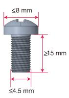
After mounting the BXP-C100 computer using the wall-mounting kit and fastening the 4 screws to fix the mounting brackets to the wall or cabinet, push the computer downwards to ensure that the device is secured firmly to the mounting surface.
