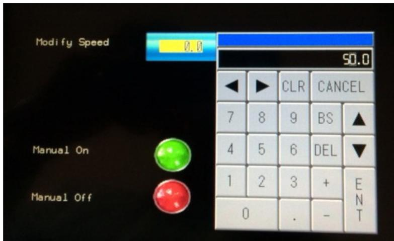
Double-click the Switch element for Manual On and change the **byManual** tag to **Set**. In the case, the Running Speed field displays 50.0.
