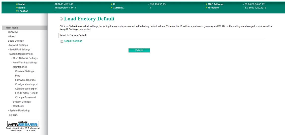
The **Load Factory Default** page is located under **Maintenance** in the **System Management** folder. Click **Submit** to reset all settings to the factory defaults. You can preserve the module's existing IP settings (i.e., IP address, netmask, gateway, WLAN profile, and all certificates) by making sure **Keep IP settings** is checked before clicking **Submit**.
