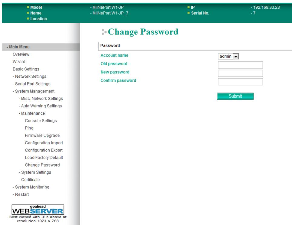
The **Change Password** page is located under **Maintenance** in the **System Management** folder. To change the password, first enter the old password in the **Old password** field. Leave this blank if the module is not currently password-protected. Enter the new password twice, once in the **New password** field and once in the **Confirm password** field. Leave these fields blank to remove password protection.
