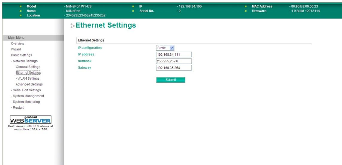
On the **Ethernet Settings** page in the **Network Settings** folder, you can modify **IP configuration, IP address, Netmask, Gateway, and Speed.**
