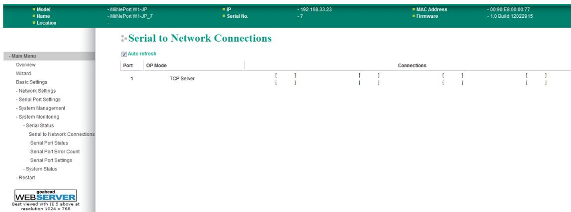
The **Serial to Network Connections** page is located under **Serial Status** in the **System Monitoring** folder. On this page, you can monitor the serial port's operation mode and host connection status.
