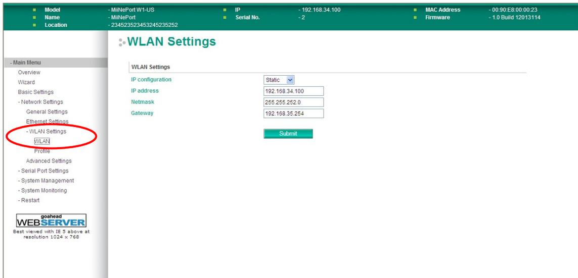
The **WLAN** page is located under **WLAN Settings** in the **Network Settings** folder. You can modify **IP configuration**, **IP address**, **Netmask**, and **Gateway** for your WLAN.
