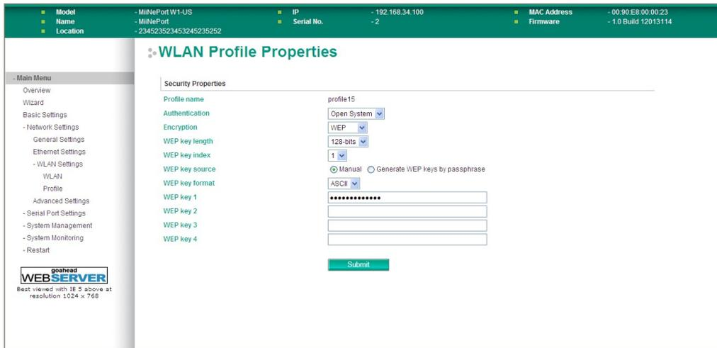
You will need to configure **Authentication** and **Encryption**. These settings must match the settings on the wireless device at the other end of the connection (such as the AP). Different settings and options are available depending on how **Authentication** and **Encryption** are configured.
