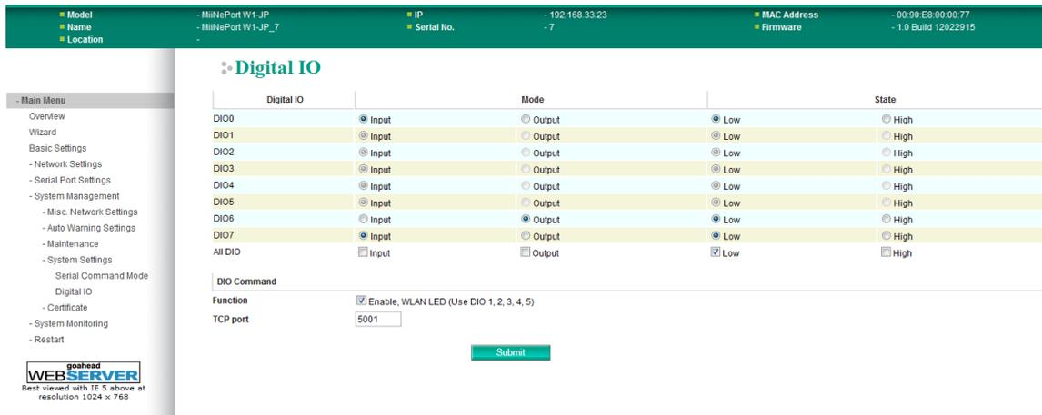
The **Digital IO** page is located under **System Settings** in the **System Management** folder. This is where you configure the 8 built-in DIO channels.
