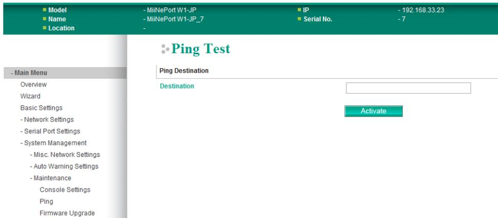
The **Ping** page is located under **Maintenance** in the **System Management** folder. It provides a convenient way to test an Ethernet connection or verify an IP address. Enter the IP address or domain name in the **Destination** field and click **Activate**. The results will be displayed immediately.
