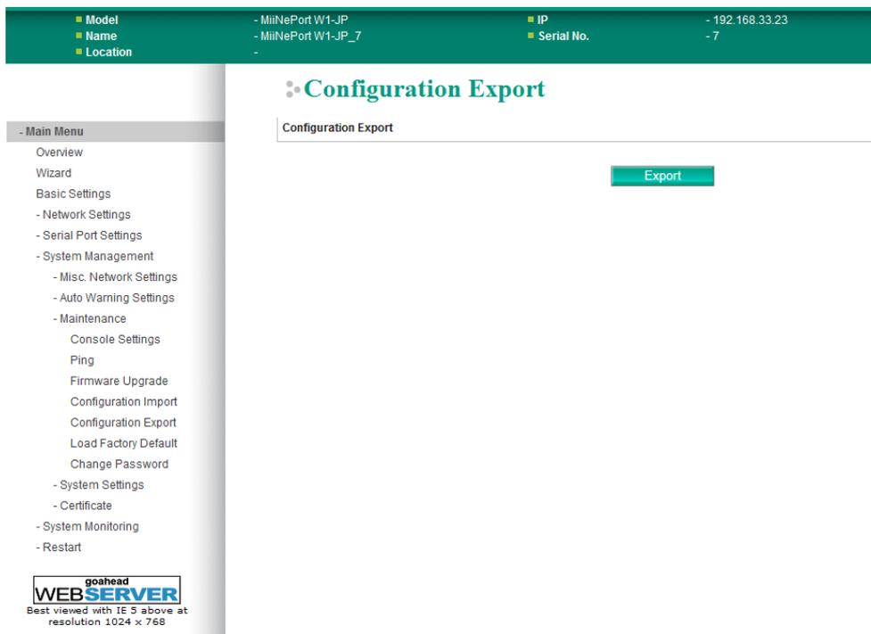
The **Configuration Export** page is located under **Maintenance** in the **System Management** folder. This is where you can save the module's current configuration to a file on the local host. Click **Download** to begin the process. A window should appear asking you to open or save the configuration text file.
