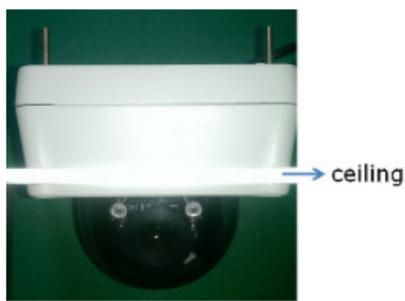
**NOTE** Because of the anti-vibration design, for onboard environments 8 kgf-cm torque is required for all mounting screws.
