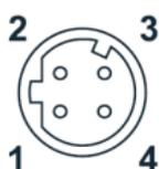
**NOTE** To connect the VPort P16-2MR series to the network, use an Ethernet cable with a D-code M12 connector and an M12 PoE switch or RJ45 PoE switch.
