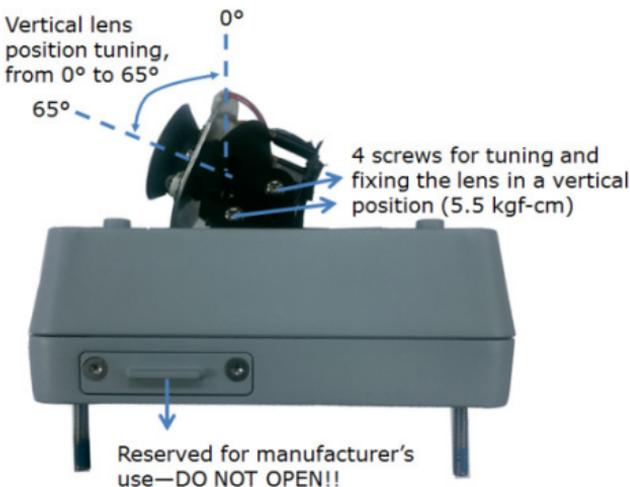
Vertical lens position tuning, from 0° to 65°
