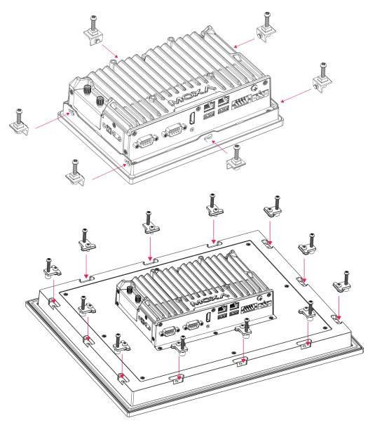
Use a torque of 5 kgf-cm to secure the mounting screws to fasten the panel-mounting kit onto the wall.
