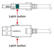
Every time you plug in and plug out the cable from the host computer, always press both latches and then plug the connector into the USB sockets on your computer or vice versa.
