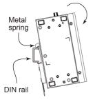
**STEP 2:** Press the UPort<sup>™</sup> 400A towards the mounting rail until it snaps into place.
