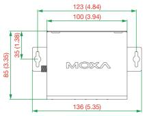
The mounting kit is 2 mm in height, and the two centers of the mounting kit on each plate is 163 mm (UPort 407A) and 123 mm (UPort 404A) apart.
