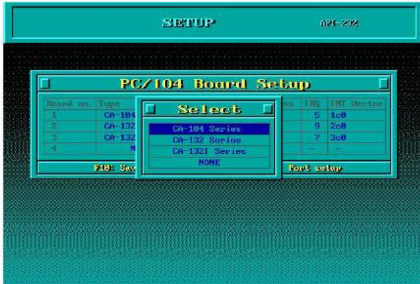
3. You must set the Port No., I/O Address, IRQ, and INT Vector properly. These settings must match your module's hardware configuration.
