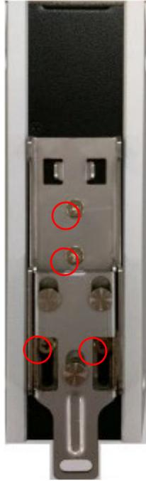
2. Remove the two screws on the rear panel.
