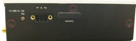
6. Remove the two screws on the bottom panel.
