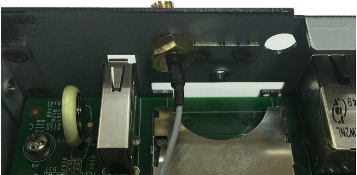
16. Secure the antenna connectors to the cover using a locking washer and nut as shown below:
