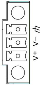
The UC-8100-ME-T has a 3-pin terminal block for a 12 to 36 VDC power input.
