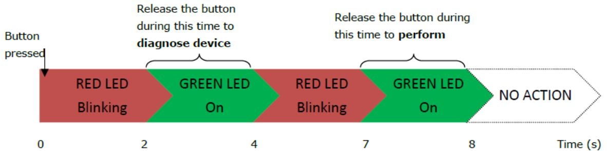
The LED indicators behave differently when diagnosing a device failure compared to performing a firmware restoration. See the following table for details:
