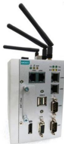
**NOTE** The MC-1121-E4-T-US model is C1D2 certified with the wireless module. The other models do not use the wireless module and hence are C1D2 certified without the wireless module.
