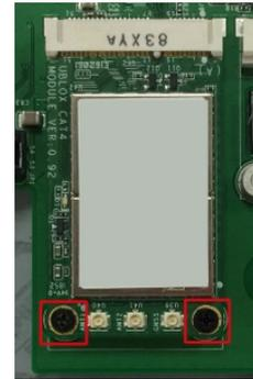
5. Connect the antenna cables to the antenna connectors.
