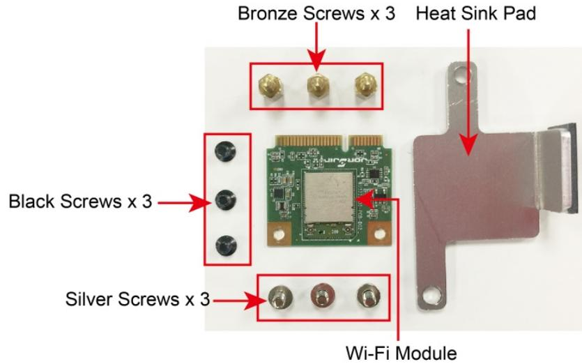
Follow these steps to install the Wi-Fi module for the UC-8220 Series.
