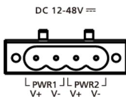
Connect the power jack (in the package) to the UC-8200 Series' DC terminal block (located on the top panel), and then connect the power adapter. It takes about 30 seconds for the system to boot up. Once the system is ready, the Power LED will light up. Both models support dual power inputs for redundancy.
