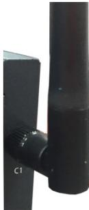
There are two cellular antenna connectors (C1 and C2) on the front panel of the UC-8220 Series. In addition, a GPS connector is provided for the GPS module. All three connectors are of SMA type. Connect the antennas to these connectors as shown below.
