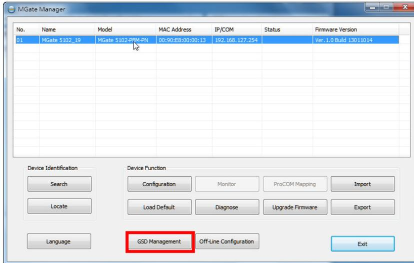
To add a GSD file, click **Add** and then assign the path where the GSD file is located. To delete a GSD file, select the GSD file and then click **Remove**.
