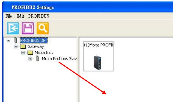
To add the device to the PROFIBUS network shown in the right panel above, drag the device from the left panel and drop it into the right panel. The device will then be shown beneath the network icon depicted in the right panel.
