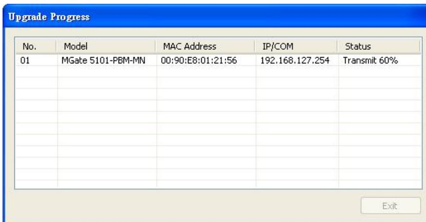
Once the firmware has been successfully written to the unit, click **Exit** to close the Upgrade Firmware window. MGate Manager will automatically execute a Broadcast Search to all MGate units on the LAN. Your MGate should reappear in the list of units.
