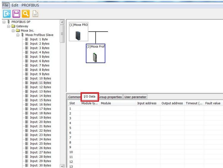
Drag the proper I/O module from the left panel to the right panel to complete the configuration.
