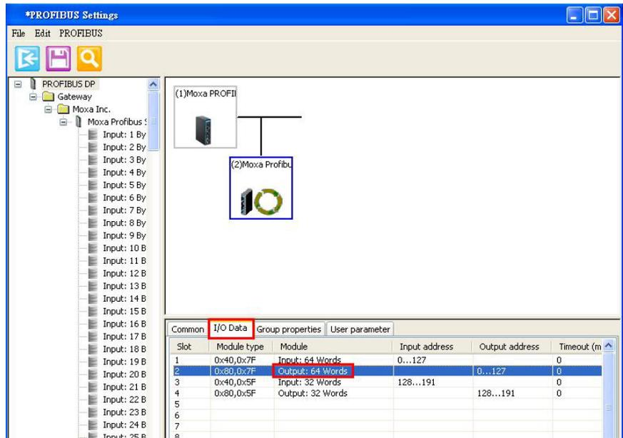
To remove the I/O modules, select the I/O module and right-click **I/O module** and select **Delete I/O** or directly press the DELETE button on your keyboard.
