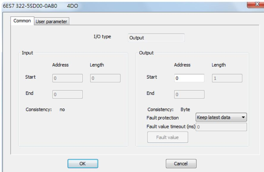
For some applications, you may want to define how to deal with the PROFIBUS output when the Modbus TCP side is not working properly. This is defined as the “Fault value”. The MGate provides a setting for each PROFIBUS I/O module to handle this kind of situation.
