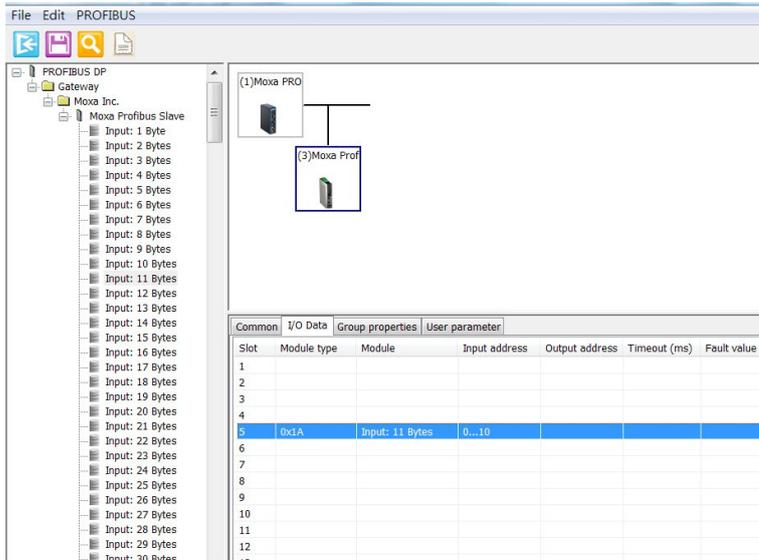
At this point, you can configure device parameters, including the slave address and I/O modules. To configure each I/O module in detail, double click the I/O module to display the configuration dialog. In the dialog box, configure the internal memory address Offset and Fault values. To configure these parameters, refer to the Data Exchange Between PROFINET and PROFIBUS and Fault Value Configuration in the PROFIBUS Output Module sections.
