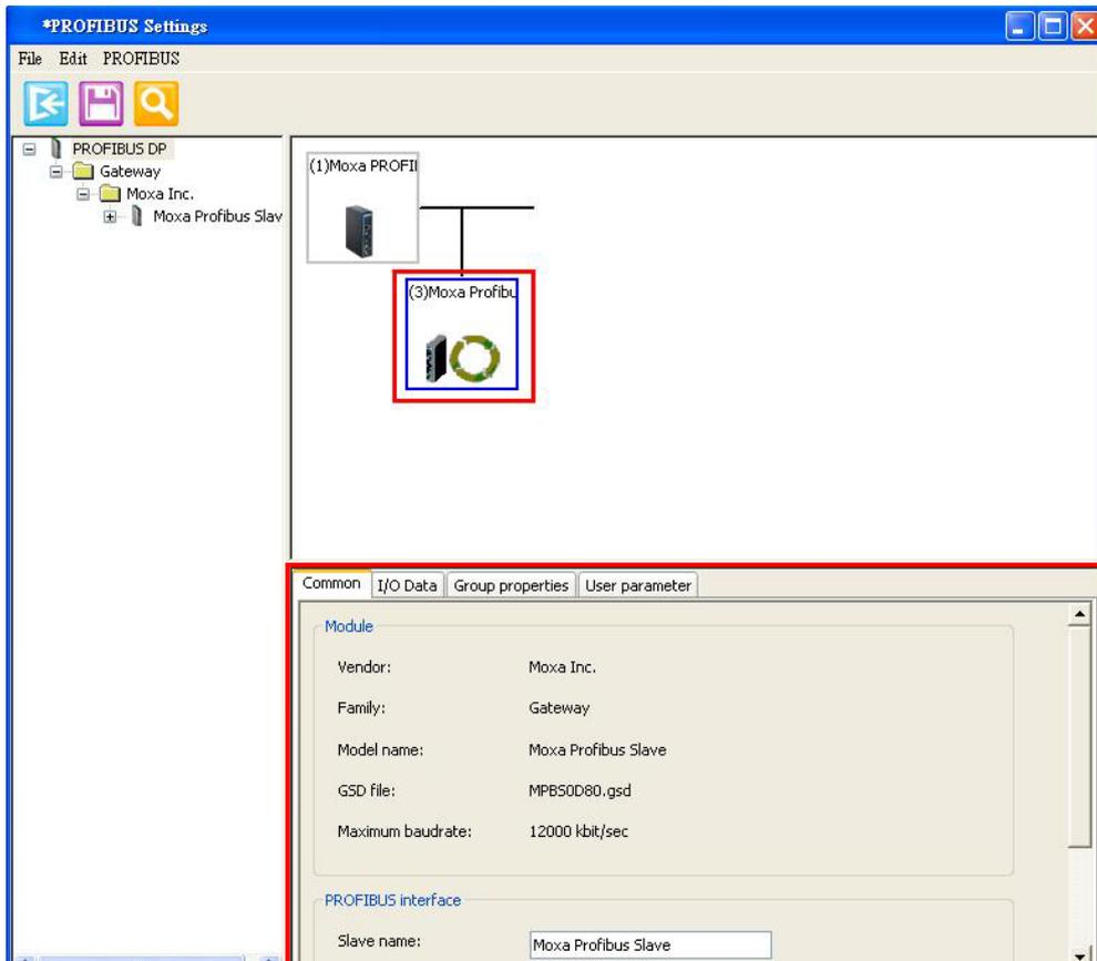
**Step 5: Configure the I/O module for the specific PROFIBUS slave device you want to access.**
