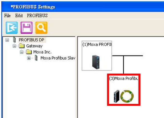
To remove the device from the PROFIBUS network (depicted at the top of the right panel in the figure above), right-click on the device and select **Delete device** or directly press the DELETE button on your keyboard.
