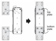
**STEP 2**—Mounting the EDS-P506E-4PoE Series on the wall requires 4 screws. Use the EDS-P506E-4PoE Series, with wall mount plates attached, as a guide to mark the correct locations of the 4 screws. The heads of the screws should be less than 6.0 mm in diameter, and the shafts should be less than 3.5 mm in diameter, as shown in the figure on at right.
