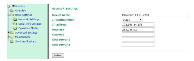
You must assign a valid IP address to the module before it will work in your network environment. Your network system administrator should provide you with an IP address and related settings for your network. The IP address must be unique within the network; otherwise the module will not have a valid connection to the network. First time users can refer to **Chapter 5: Initial IP Address Configuration** for more information.
