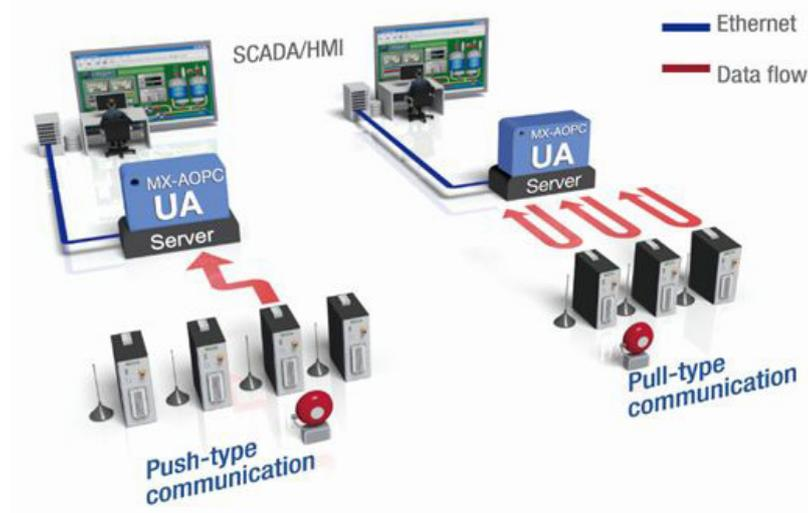
With Moxa's powerful MX-AOPC Server support, communications efficiency between ioLogik 2500-GPRS/HSPA devices and the central SCADA are substantially improved. Moxa's MX-AOPC Server's non-polling communications architecture supports the standard OPC protocol, but instead of requiring the SCADA to poll edge devices it allows edge devices to actively push communications to the central HMI/SCADA system, empowering the network with real time I/O updates while substantially cutting network overhead.
