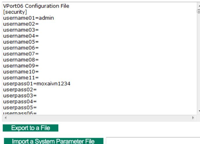
**NOTE** The system parameter import/export functions allow the administrator to back up and restore system configurations. The Administrator can export this sys\_config.ini file (in a special binary format) for backup, and import the sys\_config.ini file to restore the system configurations of VPort IP cameras. System configuration changes will take effect after the VPort is rebooted.
