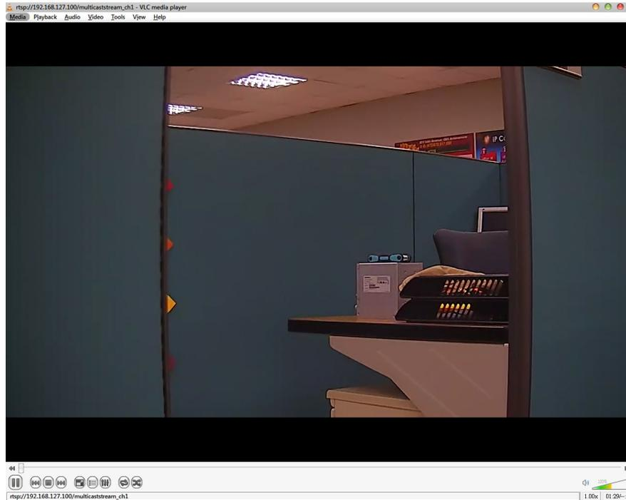
**NOTE** The video performance of the VPort may vary depending on the media players or on network performance. For example, you will notice a greater delay when viewing the VPort’s live stream from the VLC player compared to viewing it directly from the VPort’s home webpage. Also, additional delays could happen if viewing the VPort’s live stream from the VLC player over a router or Internet gateway.
