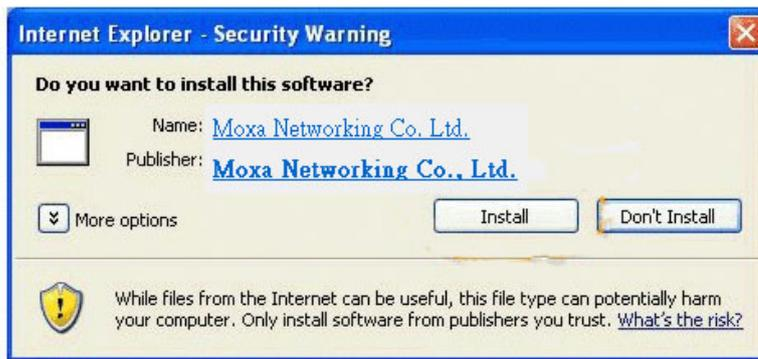
**NOTE** For Windows XP SP2 or above operating systems, the ActiveX Control component will be blocked for system security reasons. In this case, the VPort's security warning message window may not appear. Unlock the ActiveX control blocked function or disable the security configuration so that you can install the VPort's ActiveX Control component.
