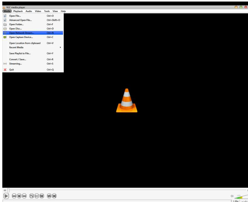
**Step 2:** When the following pop-up window appears, type the URL in the input box. E.g., type **rtsp://<VPort's IP address>[:<RTSP Port>]/live?pf=<profile ID>&pt=udp**
