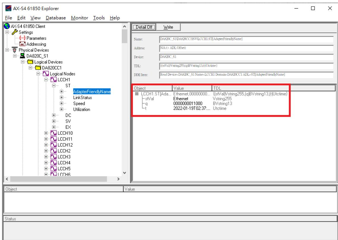
4. To view the status of the expansion card (PRP/HSR), select **DataSet<sup>[3]</sup>** or **Data Object** under **Logical Nodes<sup>[4]</sup>** to obtain the value from the MMS server.
