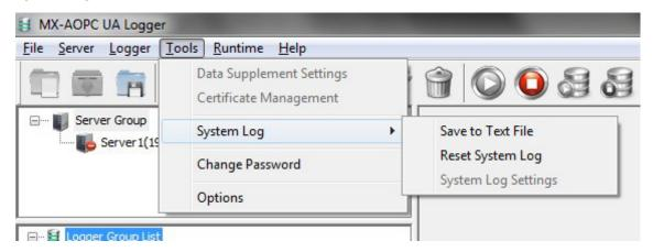
> Save to Text File: Save the MX-AOPC UA Logger's system log to a text file. You will be required to enter a password (default password = moxa).
