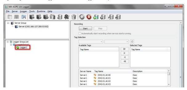
A yellow light next to the logger name shows that the logger setting is not correct. Check the settings of the logger, and then confirm the database or spreadsheet settings again.
