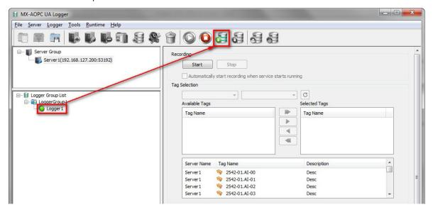
A red light next to the logger indicates that the logger is recording.
