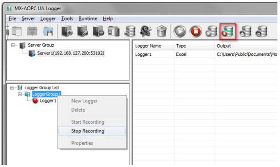
8. To check the recorded data, stop the runtime service and click the data folder of the logger. Open the data file in the folder to check the recorded data.
