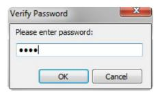
> **Reset System Log:** Reset the MX-AOPC UA Logger's system log. You will be required to enter a password (default password = moxa).
