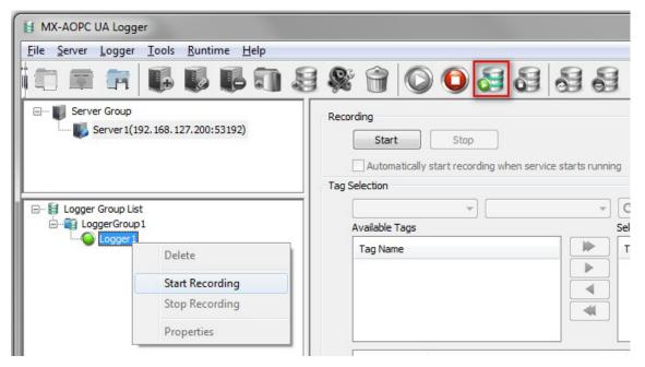
7. To stop recording, right click on the logger group or the logger and then click **Stop Recording** in the pop-up menu, or click the logger group or the logger to select it and then click the **Stop Recording** icon on the Quick Launch toolbar.
