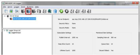
5. Once the server is connected, you will not be allowed to change the server connection settings. To change the server connection settings, click the **Disconnect** icon to disconnect the MX-AOPC UA Server, and then click the **Properties** icon to change the server connection settings.
