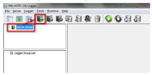
2. Select the **Local Server** option if MX-AOPC UA Server and MX-AOPC UA Logger are installed on the same computer. Otherwise, select the **Remote Server Endpoint** option and paste in the Server Endpoint from the previous step. Type in the MX-AOPC UA Server's password and then click **Next**.
