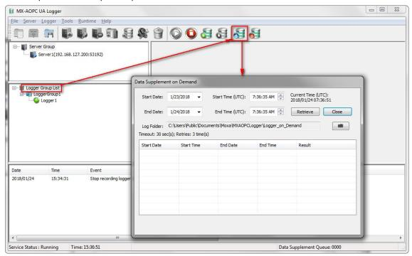
4. Click the **Retrieve** button to retrieve lost data in the defined period. The pink and gray flashing light shows that the logger is performing the data supplement process.
