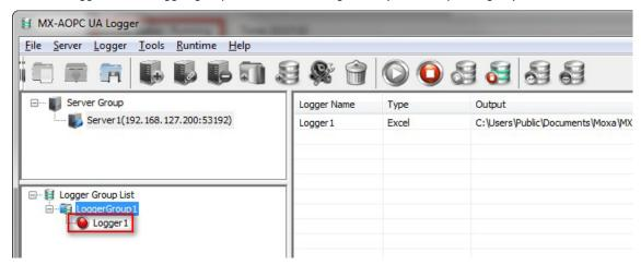
To record a specific logger, right click on the logger and then click **Start Recording** in the pop-up menu, or click the logger to select it and then click the **Start Recording** icon on the Quick Launch toolbar.
