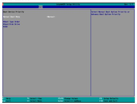
4. Select USB disk and then press "+" to move it to the first boot device position.
