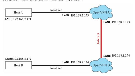
2. On machine OpenVPN A, modify the remote address in configuration file /etc/openvpn/tun.conf.
