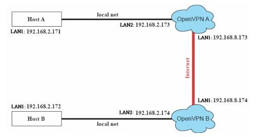
2. The configuration procedure is almost the same as for the previous example. The only difference is that you will need to comment out the parameter **up** in **/etc/openvpn/tap0-br.conf** of OpenVPN B.
