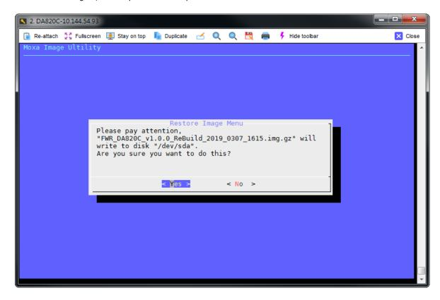
Press OK and wait for restore image process. If the process was finished, you can select to reboot, and remove the USB drive after the computer has been powered off, and jump to Step4.
