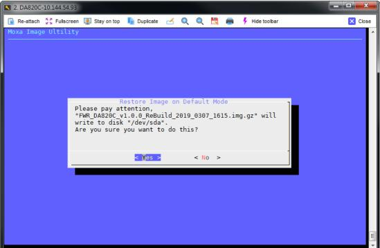
Press OK and wait for restore image process. If the process was finished, you can select to reboot, and remove the USB drive after the computer has been powered off, and jump to Step4.
