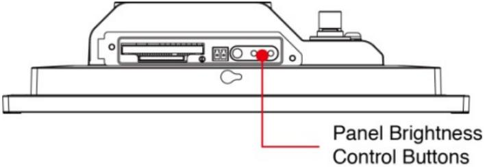
The display-control buttons can be used as described in the following table:
