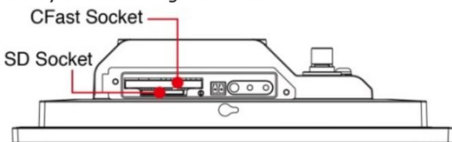
2. Insert a CFast or SD card into the respective slot using the push-push mechanism.
