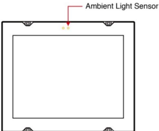
The ambient light sensor helps automatically adjust the brightness of the panel with the ambient light condition. This function is disabled by default and has to be enabled before it can be used. For details, refer to the *MPC-2121 Hardware User's Manual*.
