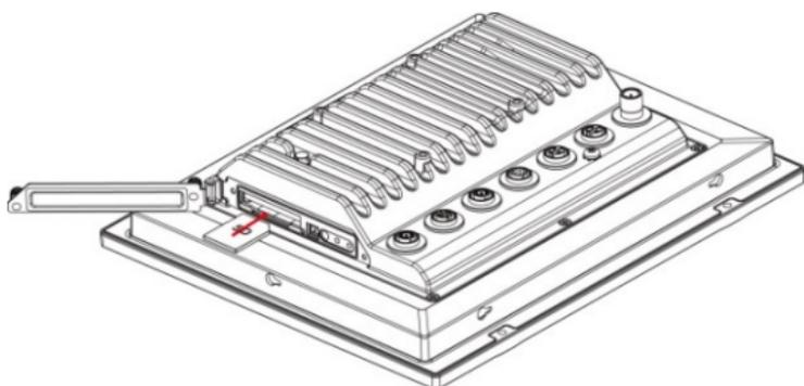
3. Reattach the cover and secure it with screws.
