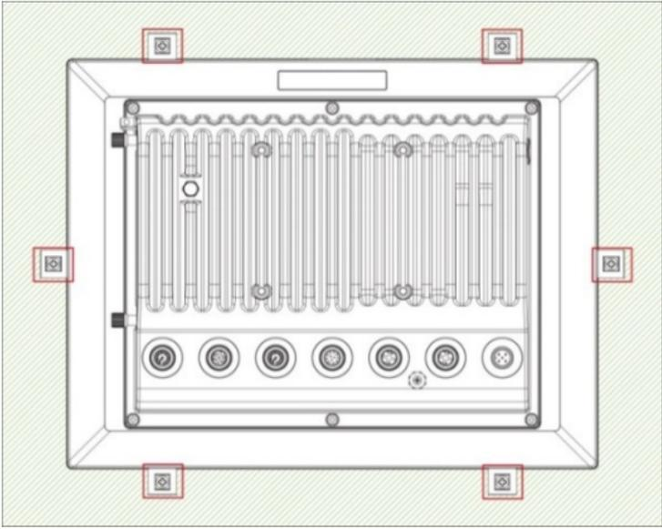
2. Use a torque of 4Kgf-cm to fasten the mounting screws and secure the panel-mounting kit units onto a wall.
