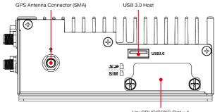
Up: SDHC/SDXC Slot x 1 Down: µSIM Card Slot x 1
