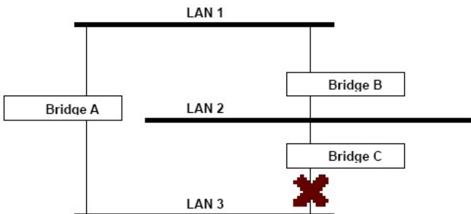
STP will determine which path between each bridged segment is most efficient, and then assigns a specific reference point on the network. When the most efficient path has been identified, the other paths are blocked. In the previous 3 figures, STP first determined that the path through Bridge C was the most efficient, and as a result, blocked the path through Bridge B. After the failure of Bridge C, STP re-evaluated the situation and opened the path through Bridge B.
