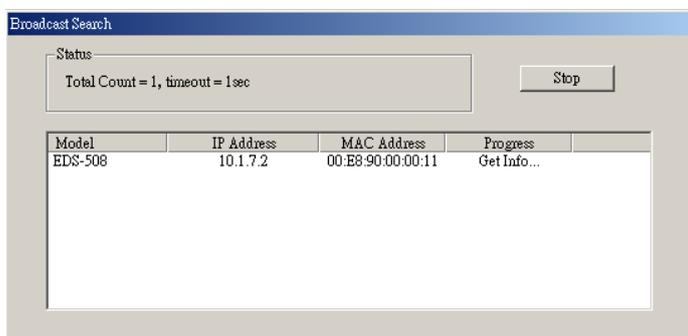
Once the search is complete, the Configurator window will display a list of all switches that were located.
