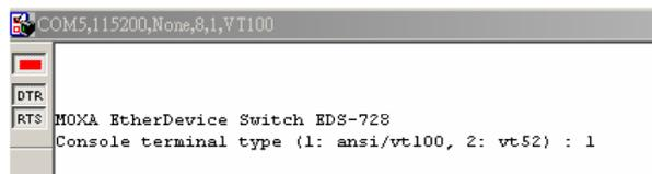
6. The Console login screen will appear. Press **Enter** to open the Account pop-up selector and then select either **admin** or **user**. Use the keyboard's down arrow to move the cursor to the Password field, enter the **Console Password** (this is the same as the Web Browser password; leave the **Password** field blank if a console password has not been set), and then press **Enter**.
