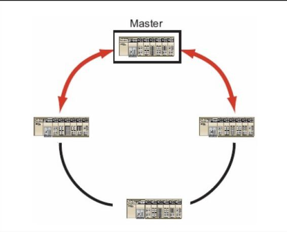
For a "Turbo Ring V2" ring, the backup segment is the segment connected to the 2nd redundant port on the master.
