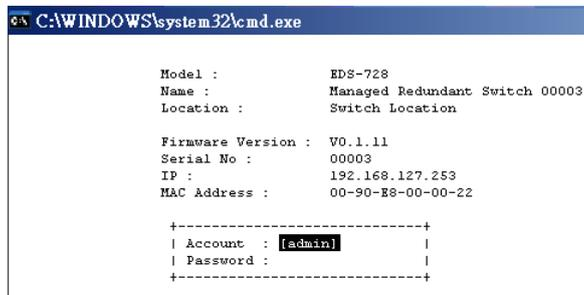
**NOTE** The Telnet Console looks and operates in precisely the same manner as the RS-232 Console.
