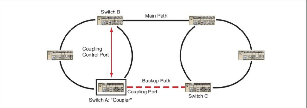
To configure the Ring Coupling function for a "Turbo Ring" ring, select two EDS-728 units (e.g., Switch A and B in the above figure) in the ring, and another two EDS-728 units in the adjacent ring (e.g., Switch C and D).
