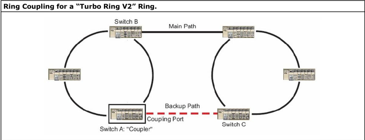
Note that the ring coupling settings for a "Turbo Ring V2" ring are different from a "Turbo Ring" ring. For Turbo Ring V2, Ring Coupling is enabled by configuring the "Coupling Port (Primary)" on Switch B, and the "Coupling Port (Backup)" on Switch A only. You do not need to set up a coupling control port, so that a "Turbo Ring V2" ring does not use a coupling control line.
