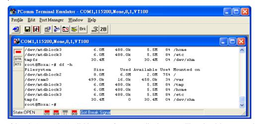
If there isn't enough "Available" space for your application, you will need to delete some existing files. To do this, connect your PC to the IA240/241 with the console cable, and then use the console utility to delete the files from the IA240/241's flash memory. To check the amount of free space available, look at the directories in the read/write directory /dev/mtdblock3. Note that the directories /home and /etc are both mounted on the directory /dev/mtdblock3.
