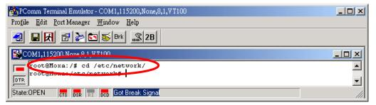
2. Type **#vi interfaces** to edit the network configuration file with vi editor. You can configure the Ethernet ports of the IA240/241 for **static** or **dynamic** (DHCP) IP addresses.
