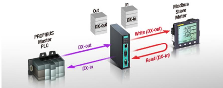
For example, let's assume two Modbus commands are mapped to two PROFIBUS modules that will be used in the PLC program. If the two Modbus commands don't get a response, then the MGate 4101-MB-PBS will send a PROFIBUS diagnostic package to the master. If the Modbus command is still failing after a dwell time of three seconds, then the MGate 4101-MB-PBS will trigger the next diagnostic package transmission.
