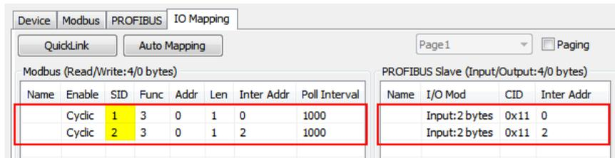
The PC runs the **Modbus Slave** simulator. Create Slave ID1 and Slave ID2 to respond to the MGate 4101-MB-PBS's polling. In this situation, the MGate is in **Normal** mode.
