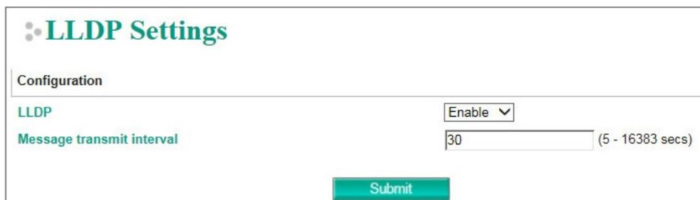
The screenshot shows the 'LLDP Settings' configuration page. It features a title 'LLDP Settings' with a gear icon. Below the title is a section header 'Configuration'. There are two fields: 'LLDP' (a dropdown menu set to 'Enable') and 'Message transmit interval' (a text box containing '30' with '(5 - 16383 secs)' to its right). A green 'Submit' button is located at the bottom center of the form.
